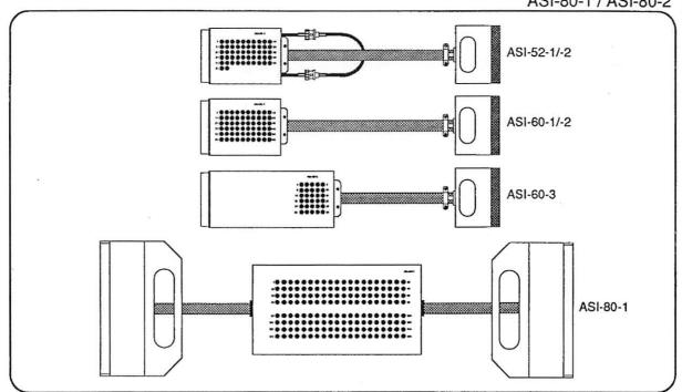
The Universal ATR Breakout Extender Cables provide access to all of the pins on the rear connector of a Collins avionics unit (equipped with a Thinline connector). The LRU can be extended from its rack in the aircraft so that signal checks and monitoring can be performed on each individual wire via the test jacks mounted in the cable chassis. Consult the matrix at the right for ASI-52-1/-2, ASI-60-1/-2/-3, and ASI-80-1 LRU compatibility.
